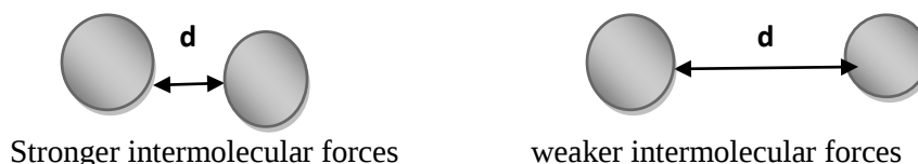
Figure 3.2 effect of distance on the size of intermolecular forces
